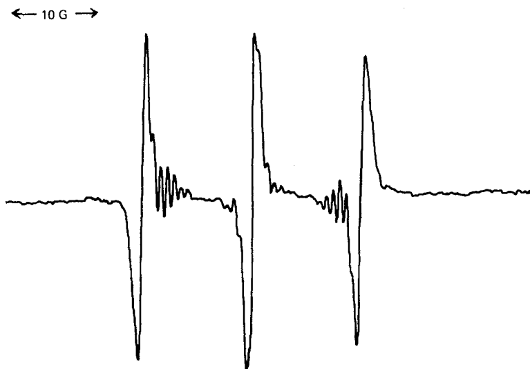
FIG. 11. ESR spectrum of the \text{Cu}(\text{eacac})_2/\text{TPB}/\text{MMA}/\text{BNO} system after reaction at room temperature for 0.5 h in acetone: [\text{Cu}(\text{eacac})_2] = 1.50 \times 10^{-3} , [\text{TPB}] = 1.50 \times 10^{-2} , [\text{MMA}] = 5.60 , [\text{BNO}] = 2.00 \times 10^{-2} mol/L.
